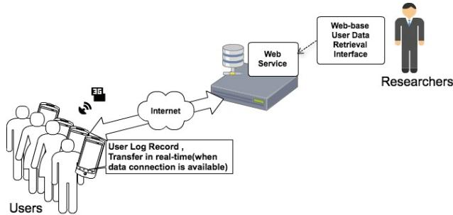
**Fig 1.** Service dataflow: user logs are saved locally using SQLite and later transmitted to a remote server when 3G/WiFi connection is available. Researcher can query the database through a web-based interface.
